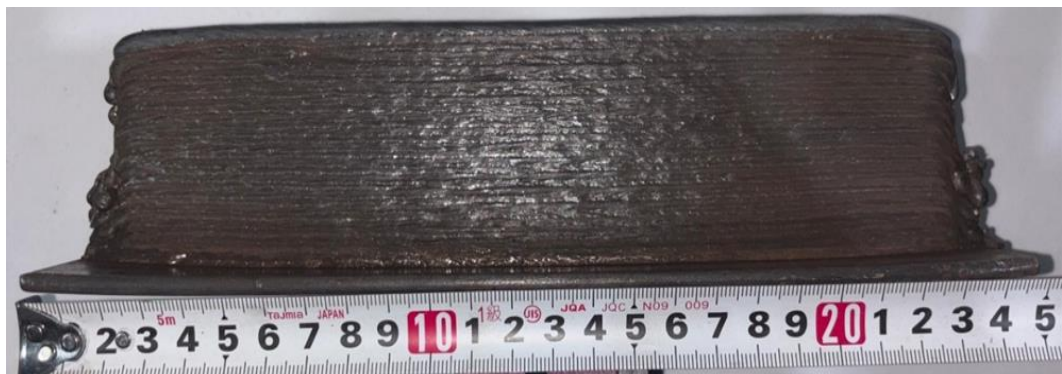
Figure 3. The WAAM single- wall structure specimen
