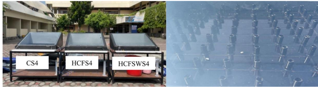
Figure 4. The placement solar still testing chamber and the cylindrical fins
