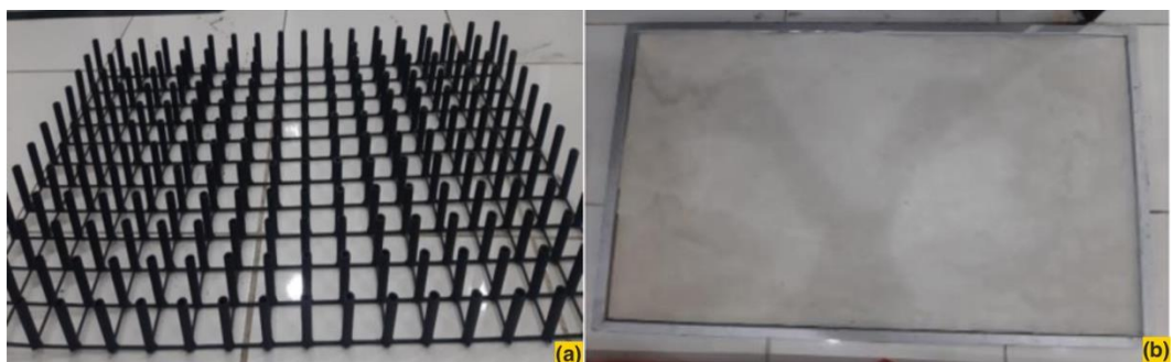
Figure 3. (a) The hollow circular fin; (b) Soybean wax PCM
