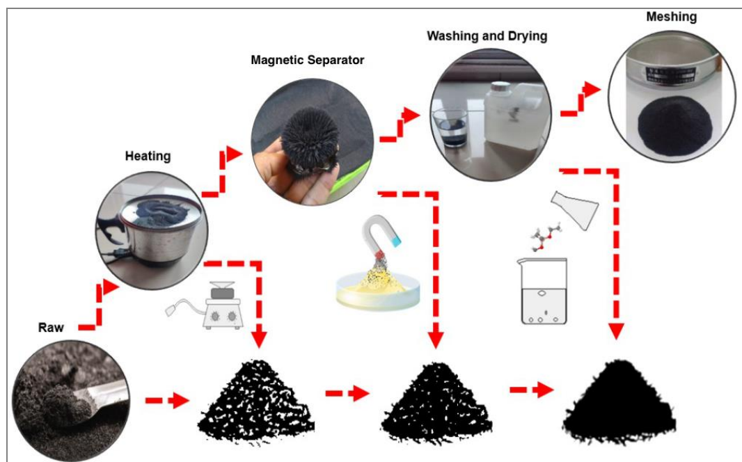
Figure 2. Separation process for mineral iron sand [32]
