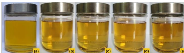
Figure 6. Snapshot of PET–EZAC pyrolysis oil products with loadings: (a) 0%; (b) 5%; (c) 10%; (d) 15%; (e) 20%
